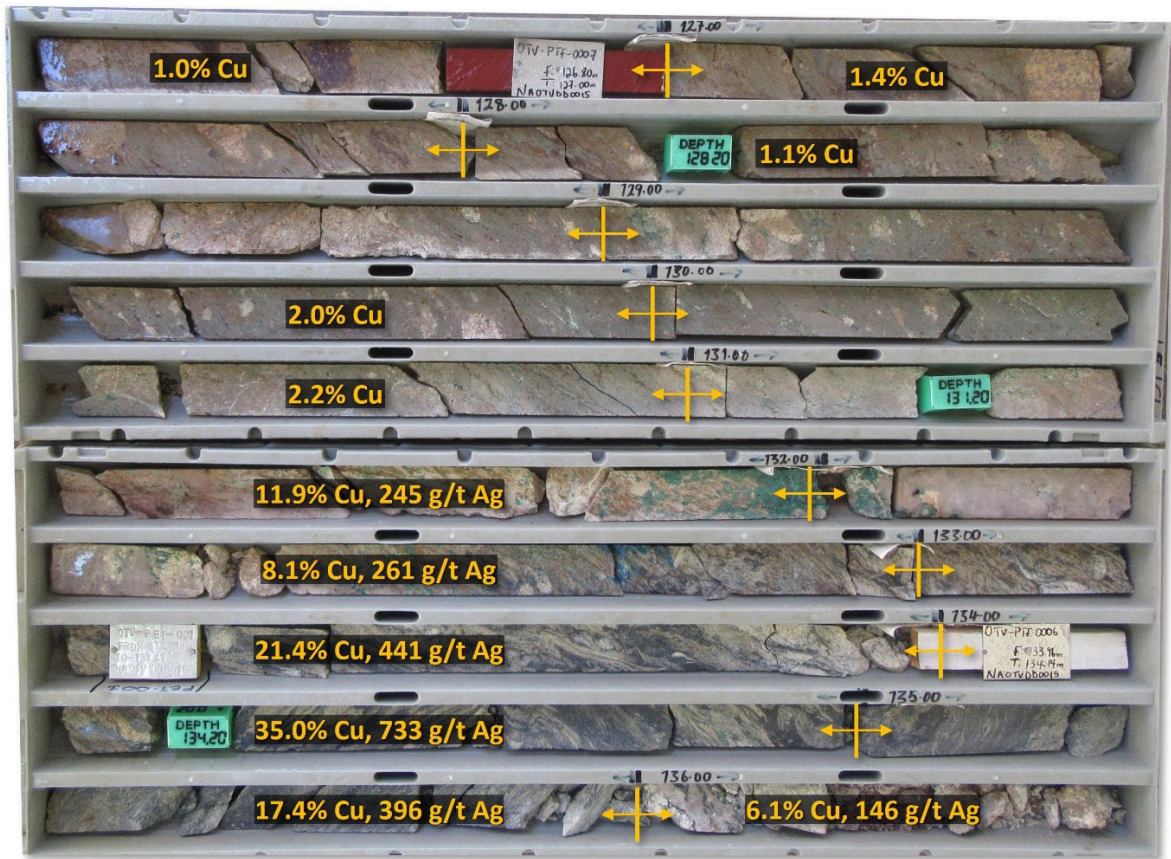
Photo 3: 'NAOTVDD0015' (126.25m - 136m), Oxide-Transition Mineralisation
