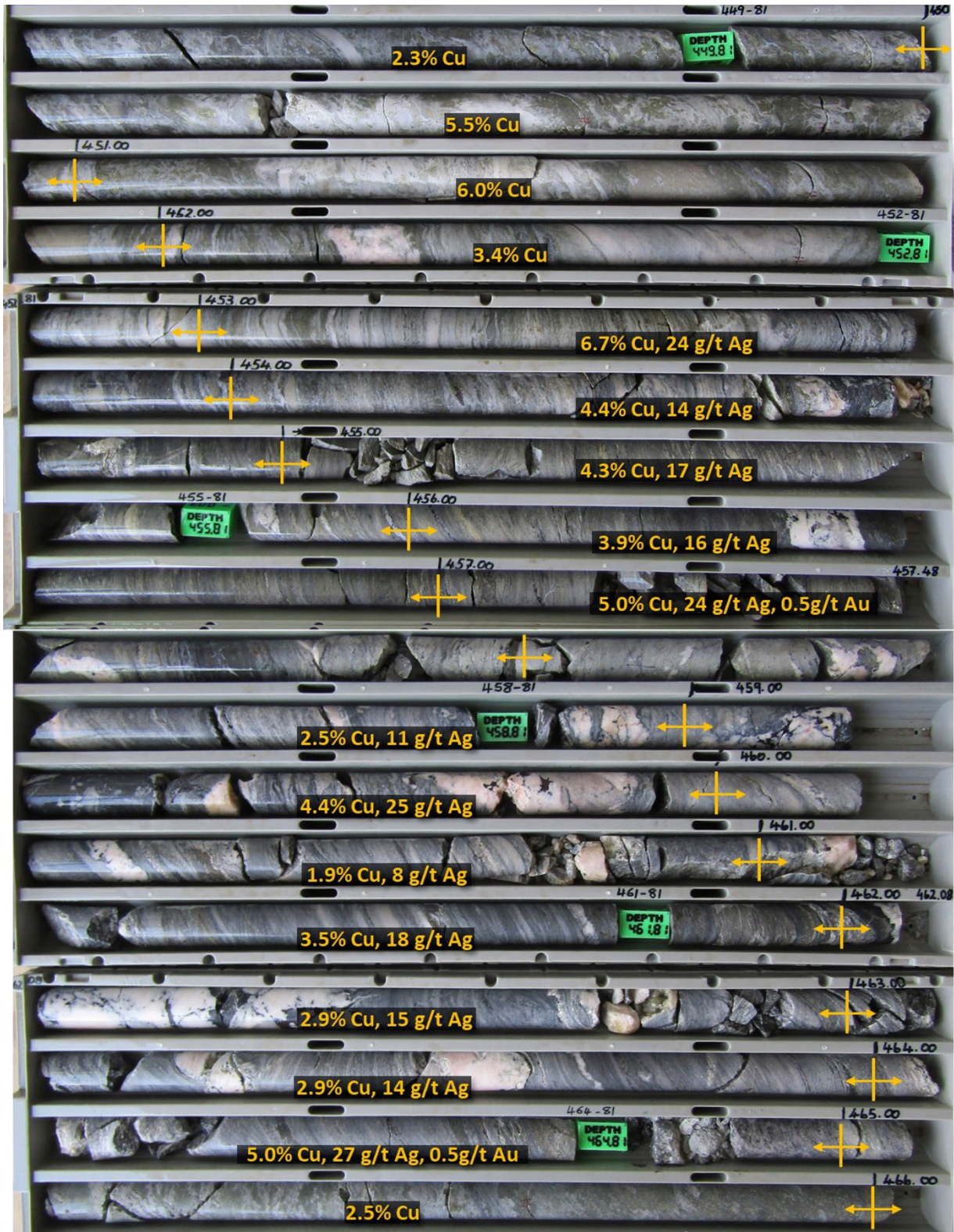
Photo 8: NANAND000011 (449m - 466.9m) Sulphide Material
