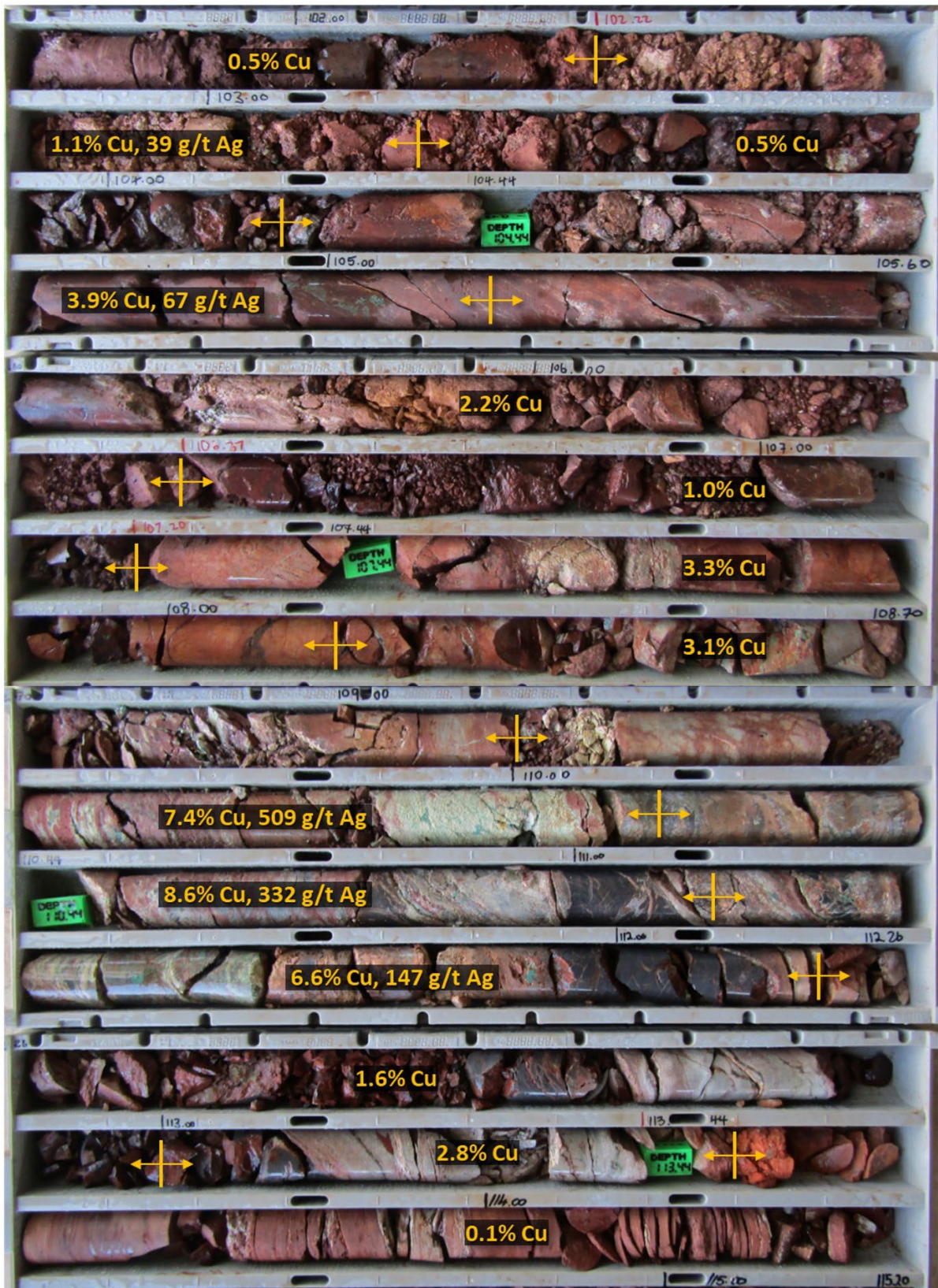
Photo 2: 'NAOTVDD00112' (108.7m - 114.3m), Oxide-Transition Mineralisation
