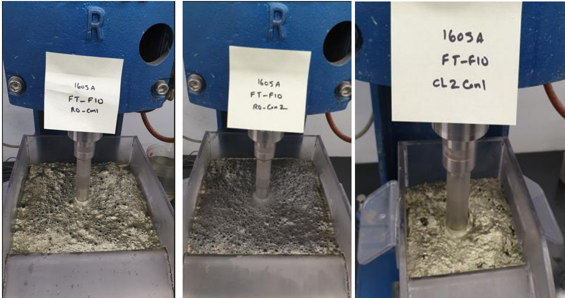
Figure 3: Copper concentrate from fresh composite, with chalcopyrite as the major copper mineral
