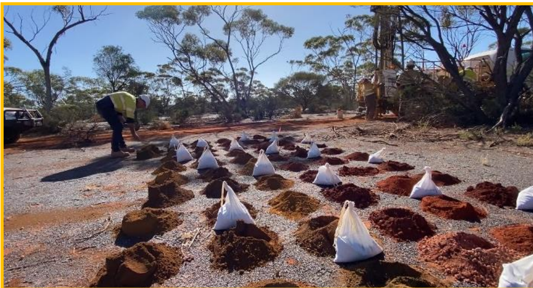
Photo 1: Executive director, Andrew Jones - Geological logging - AC drilling, El Donna Gold Project, WA.
