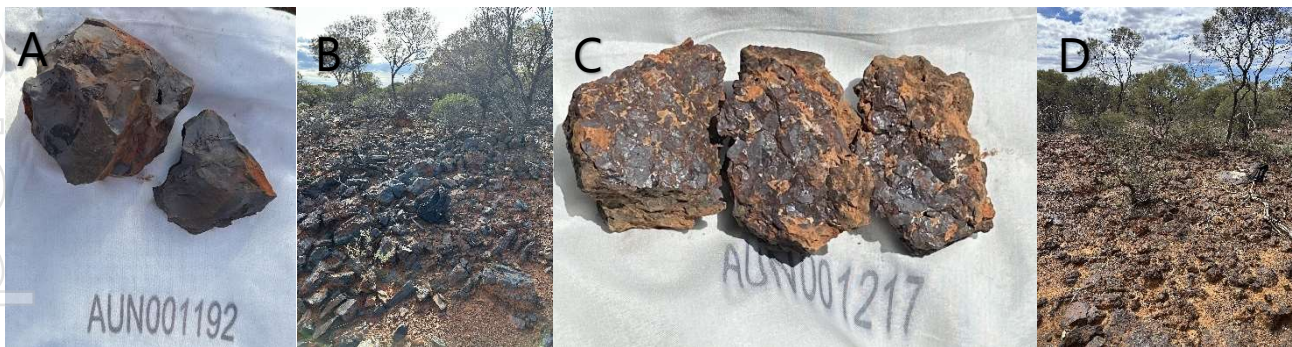
Figure 10. (A) Hematite enriched BID (Sample AUN001192 – 65.17% Fe), (B) outcropping hematite enriched BID, (C) hematite enriched capping / pisolite (Sample AUN001217 – 59.62% Fe), (D) outcropping cemented hematite pisolite potentially representing immature paleochannel iron deposits or capping.
