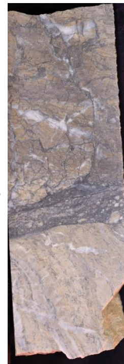
NSD058 – 283.5m the intercept, although narrow, includes very encouraging geology and structure that indicates the possibility of a Stawell-type gold system.
