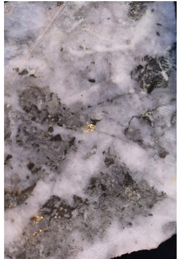
NSD057 – 108.2-109m includes multiple instances of visible gold (VG) in quartz veining. This is not typical for Stawell – and the geology, mineralisation and structure have strong similarities to the historic Mariners mines that boasted an historic production grade of ~30 g/t Au (see p. 11 for details on Mariners).
