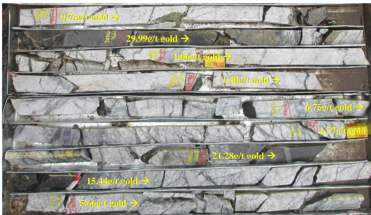
Figure 5 | FNDC028, 71.06m to 79.8m photo Interval – Assay Interval 71m to 80m averages 9m @ 7.39g/t gold within the 19m @ 3.72g/t gold reported significant intercept hosted in felsic intrusion
