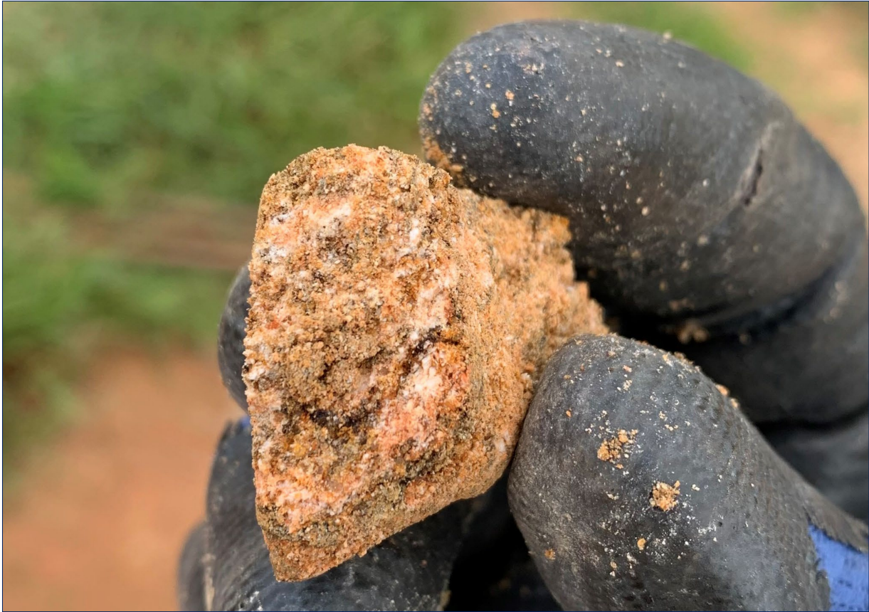
Above - Shallow mineralised interval in auger hole CAL-AUG-071 with 1m @ 1,458ppm TREO from 2m, with 31% MREO.
