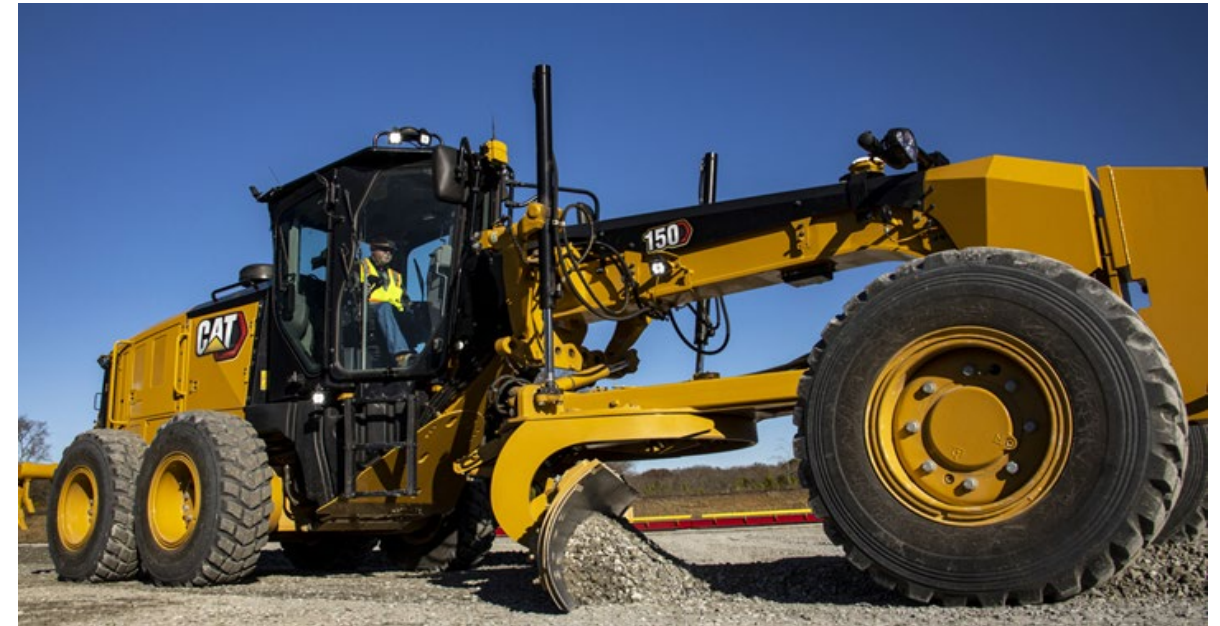
Pictured above: Caterpillar 150 - 3D Mast-less grade control - All Wheel Drive Grader
