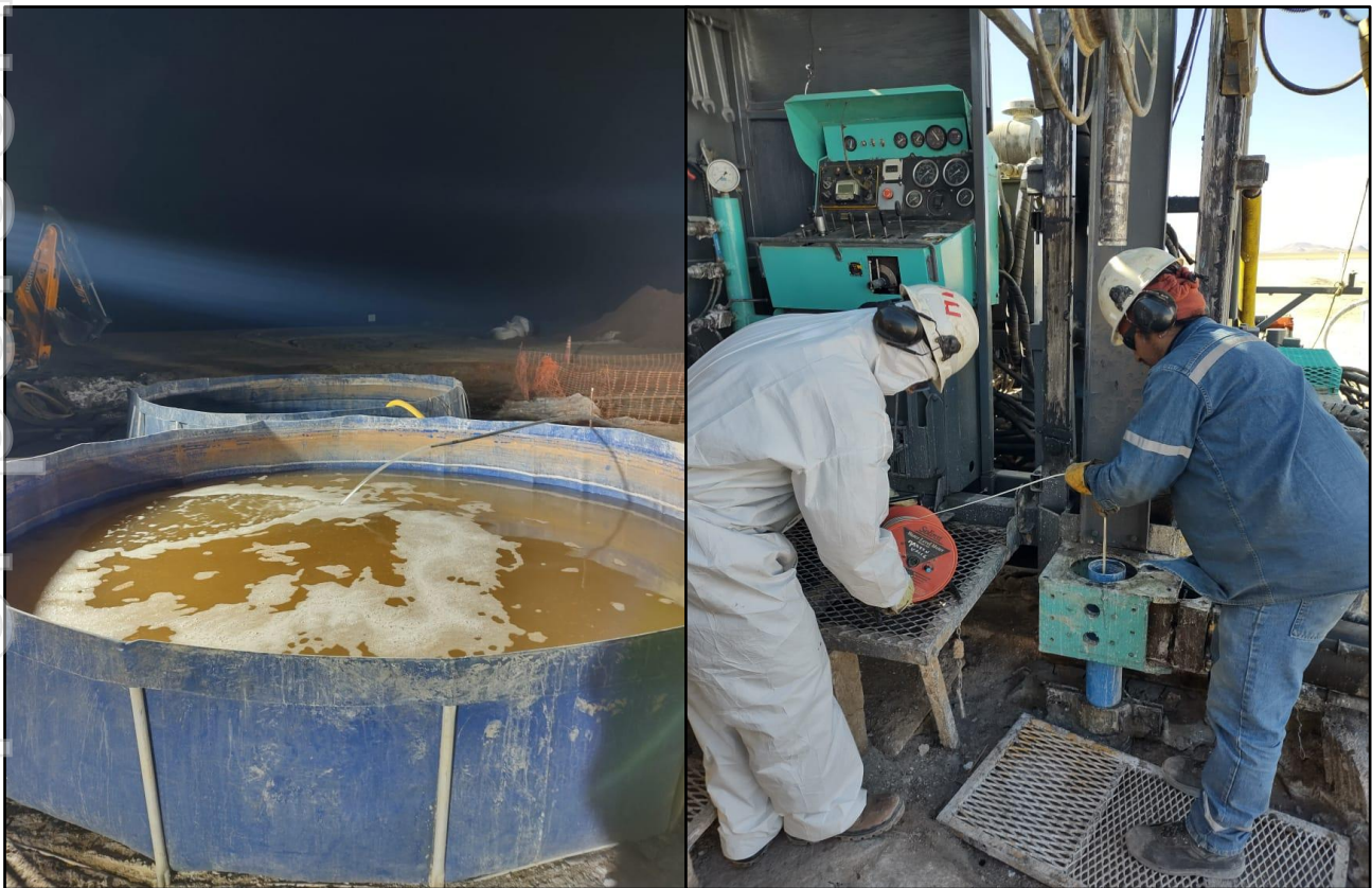
Figure 4. Showing 11,000 litre tank holding brines pumped at 2,597 litres per hour and well logger being operated.
