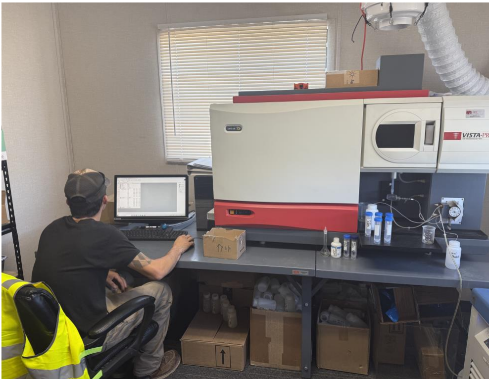
Figure 1 : Anson/A1 Green River employee trained by A1 to assay brine and lithium eluate samples using ICP (Inductively Coupled Plasma) Spectroscopy
