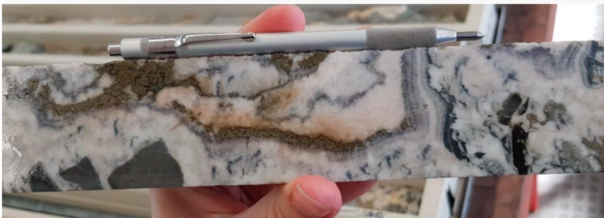
Figure 2 Epi-thermal style mineralisation, coliform banded vein breccia and Ginguro bands from historical diamond core drill hole ID PMD001. Half core shown from down hole depth 748-749m with lab assays returning 0.65g/t gold, 0.25% Arsenic and 2.2g/t silver over 1m, typical of epi-thermal systems. (picture and description - supplied by Rimfire).
