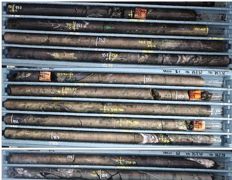
Figure 5: DD24KP1232 - Footwall structure outside known mineralisation. 7.7m @ 5.95g/t Au, 3.4% Cu, 22.2g/t Ag from 350.5m including 3.7m @ 11.3g/t Au, 4.8% Cu, 33.3g/t Ag from 354.5m. Mineralisation occurs as massive and semi massive sulphides overprinting quartz veining from 351.2m, comprised of pyrrhotite (60%) and semi massive chalcopyrite (15%) and pyrite (5%). True width of the interval is estimated to be approximately 65% of the visually logged intercept length.
