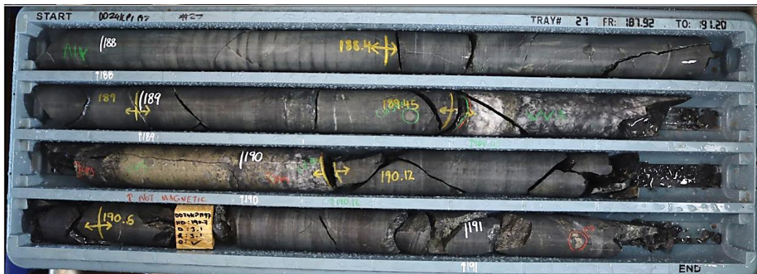
Figure 4: DD24KP1197 intersected 4.6m @ 9.2g/t Au, 0.6% Cu, 3.6g/t Ag from 189.5m including 0.7m 56.3g/t Au, 4.0% Cu, 22.1g/t Ag from 354.5m. Mineralisation is hosted within a quartz vein with prominent sulphides including 5-20% chalcopyrite, and ~5% pyrite.
