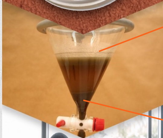
Photo 5. Laboratory HM separation via a heavy liquid
