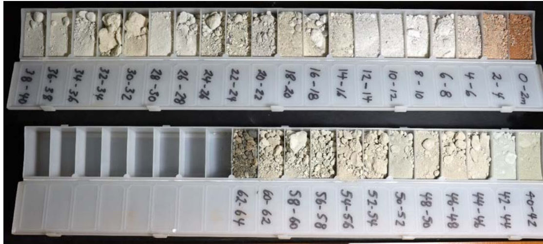
Photo 7: Drillhole 81RPH7 showing unconsolidated Algebuckina sands to 62m
