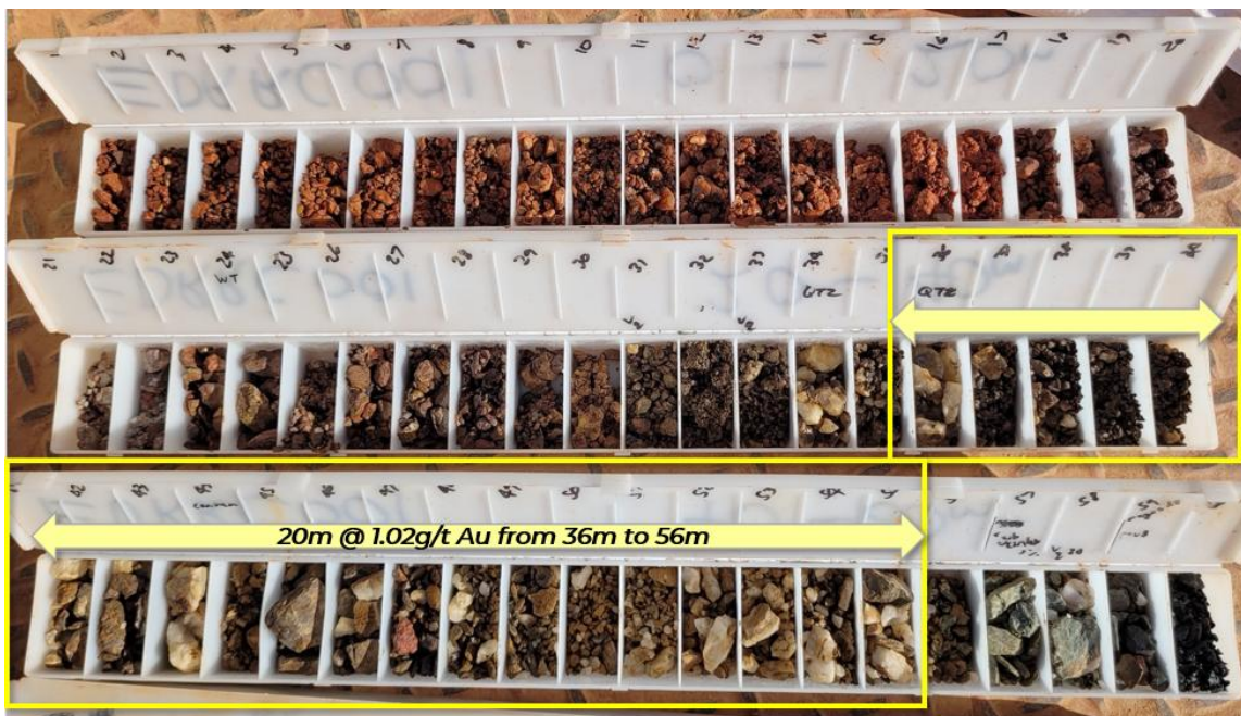
Photo 1: Chip tray showing washed 1m samples in the upper part of RC drillhole EDRRC001 and the extent of quartz iron-manganese veining within the gold intercept of 20m @ 1.02g/t Au.
