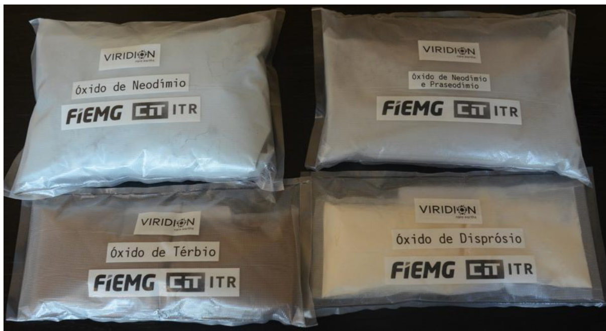
Figure 1: Recycled high-purity Nd, Pr, Dy, Tb oxides delivered to CIT SENAI ITR / FIEMG, originating from end-of-life magnets recovered in Brazil and processed at Ionic Technologies' facility in Belfast (UK).
