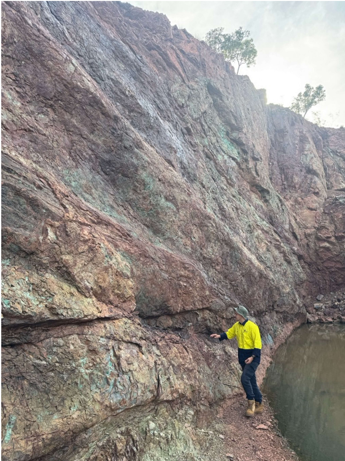
Figure 3: Jointing and shearing displayed along face of Pit 1 at the Big One Deposit
