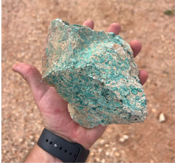
Figure 5: Kaolinite-altered trachyte dyke, disseminated malachite and chrysocolla at BOGS3 Site
