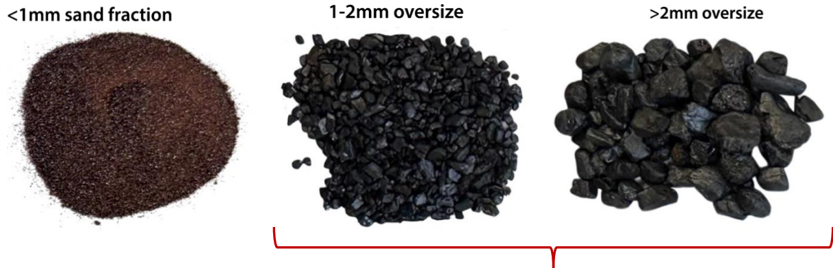
Figure 3: Representation of mineral sand particles versus oversize particles. Images of sand and oversize particles are not from Minta area – only shown to demonstrate difference in particle size.
