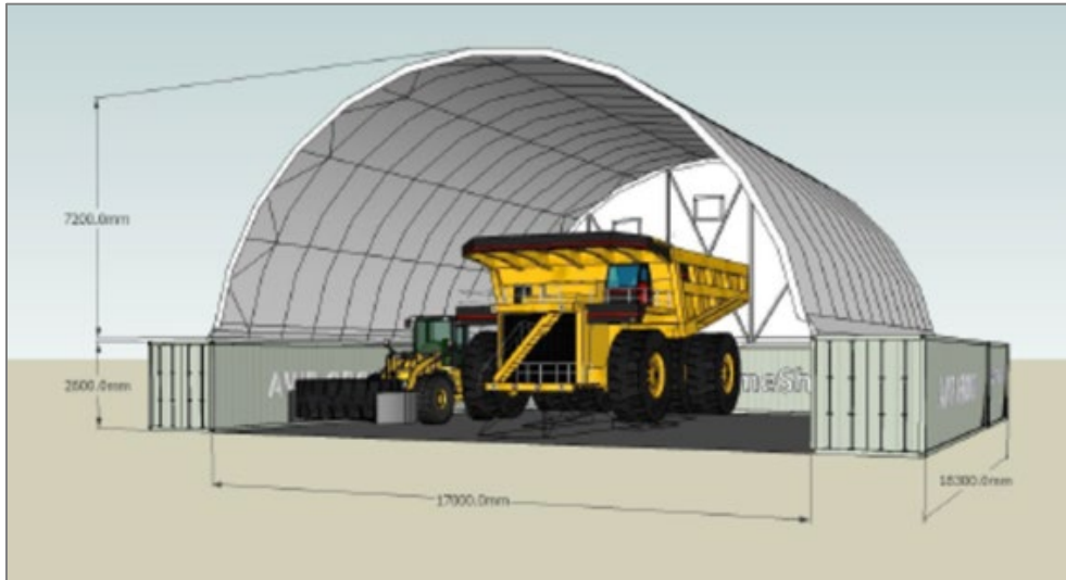
Figure 25: Example of Double-container height Haulpak workshop.
