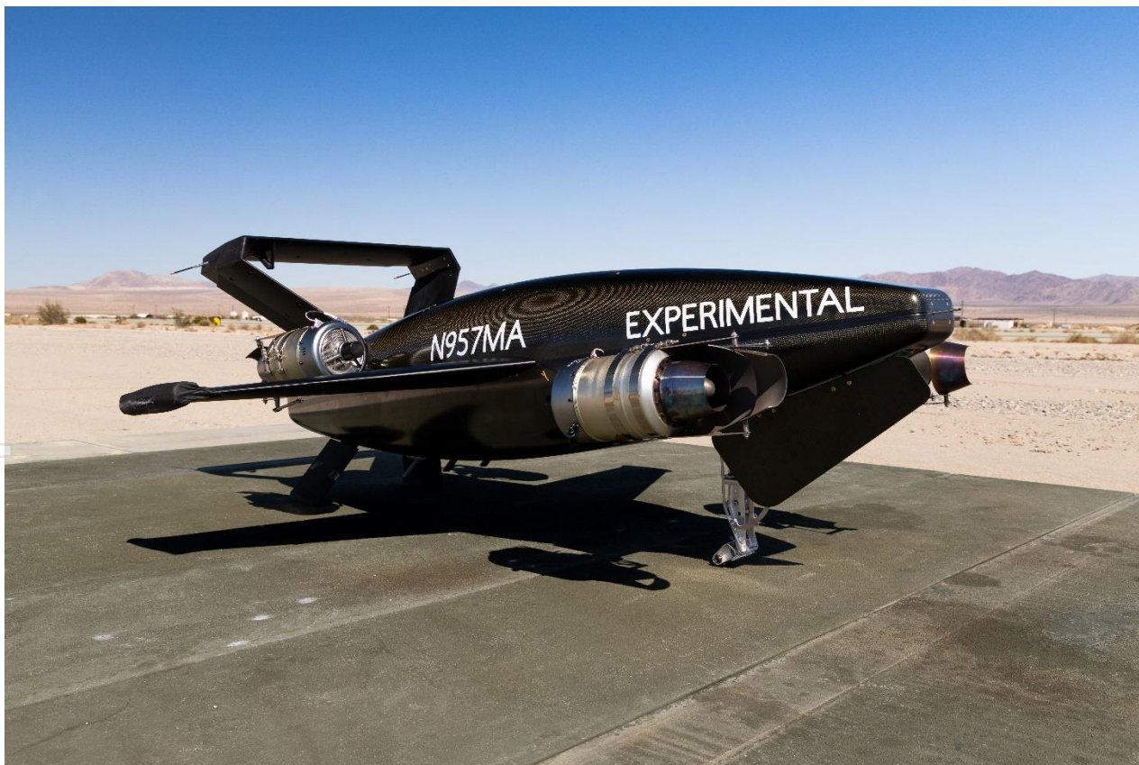
The Mayman Aerospace RAZOR Platform, Utilising 4 Micro Gas Turbines
