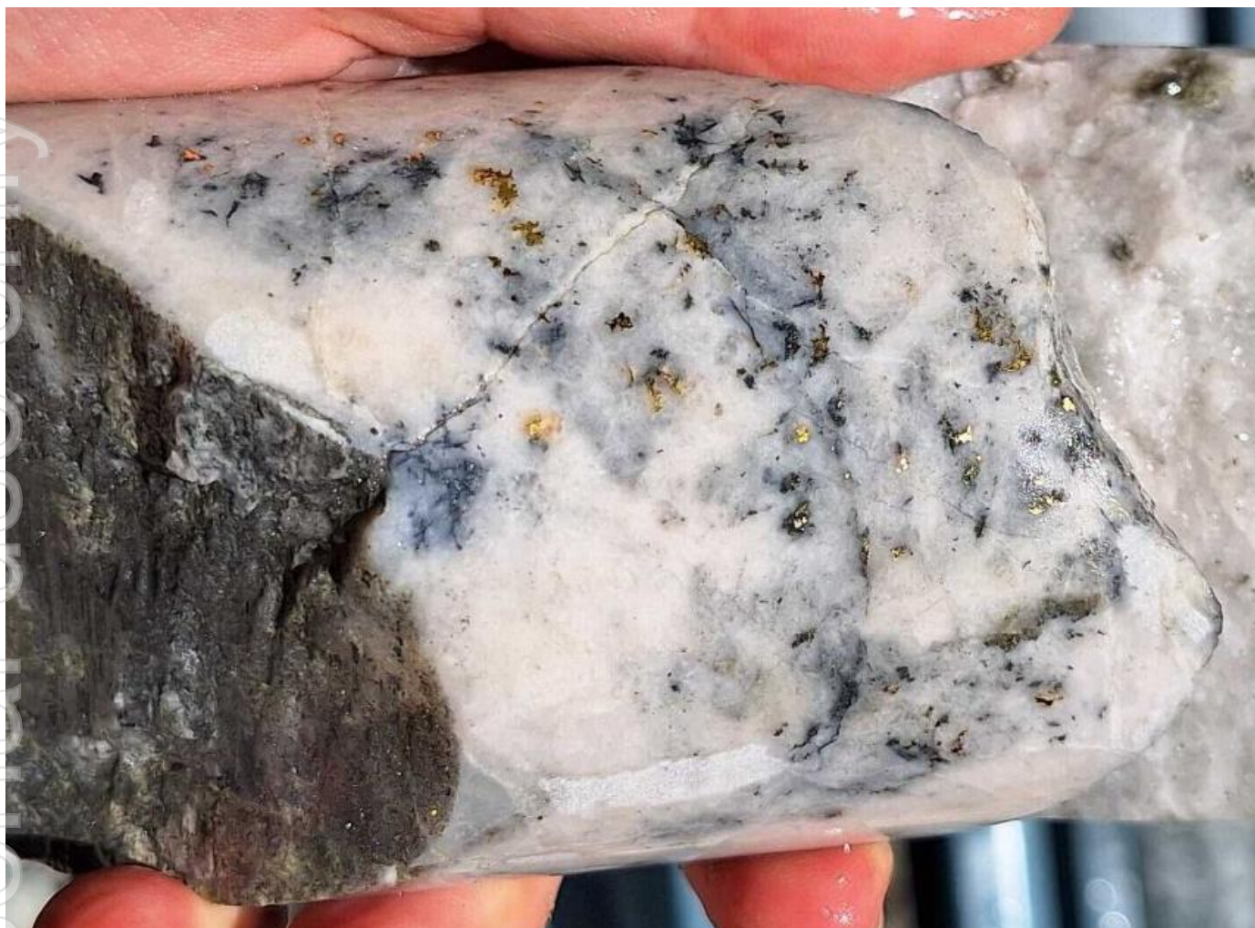
Figure 1: SDDSC161 intercept: 0.2 m @ 4,700 g/t Au and 0.26% Sb from 511.3 m showing abundant visible gold in a quartz-carbonate-stibnite vein. Part of a wider zone grading 3.4 m @ 466.4 g/t AuEq (466.0 g/t Au, 0.2% Sb) from 508.4 m. Core diameter is 63.5 mm.
