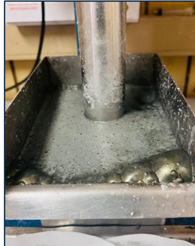
Typical Flotation test producing Rougher concentrate
