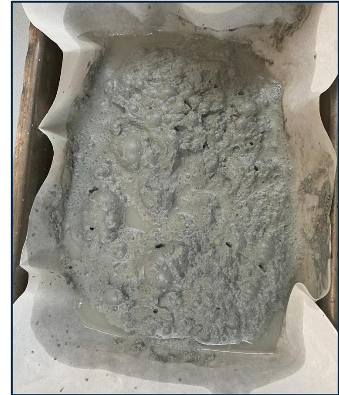
Rougher concentrate from laboratory flotation test
