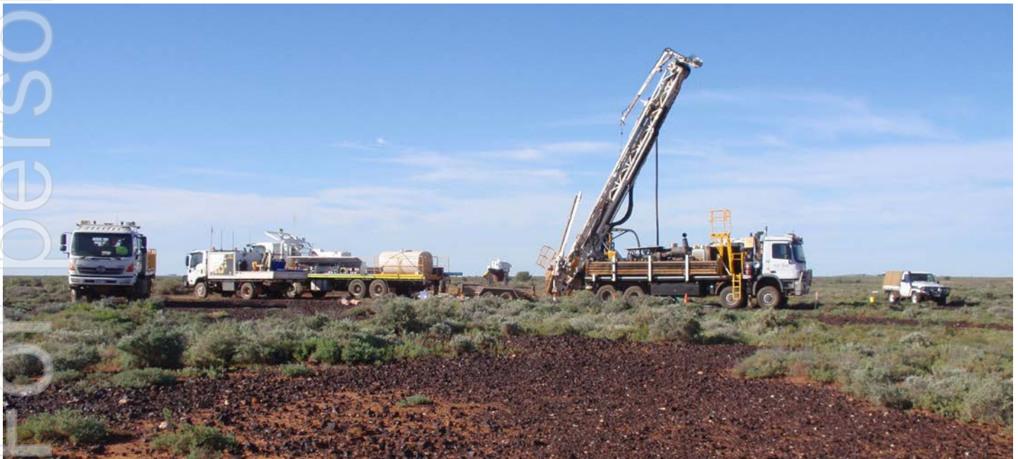
Figure 4 Drilling during 2023 of the copper anomalous gossan outcrop (dark brown ironstone scattered in the foreground) at the Johnson Dam prospect. The mineralised zone intersected dips at approximately 45 degrees east, beneath the position of the drilling rig.
