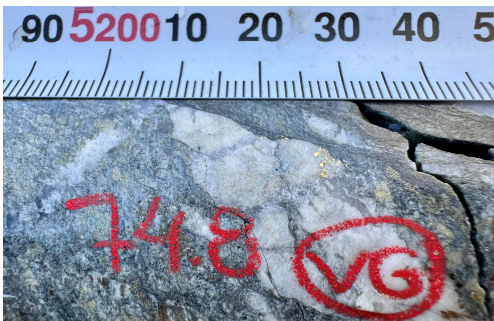
Figure 1: Visible gold intersected in hole 25PGOGC036A at 74.8m depth. Trace amounts (<0.1%) of disseminated native gold were reported from an ~5cm wide zone at 74.8m depth within an ~0.55m wide quartz-carbonate vein (see Figure 3 for further context). Visible gold was only logged along the upper contact of this vein and assays are pending for this entire interval, which are expected in July 2025. Note: visual estimates of mineral abundance should never be considered a proxy or substitute for laboratory analyses where concentrations or grades are the factor of principal economic interest. Visual estimates also potentially provide no information regarding impurities or deleterious physical properties relevant to valuations.
