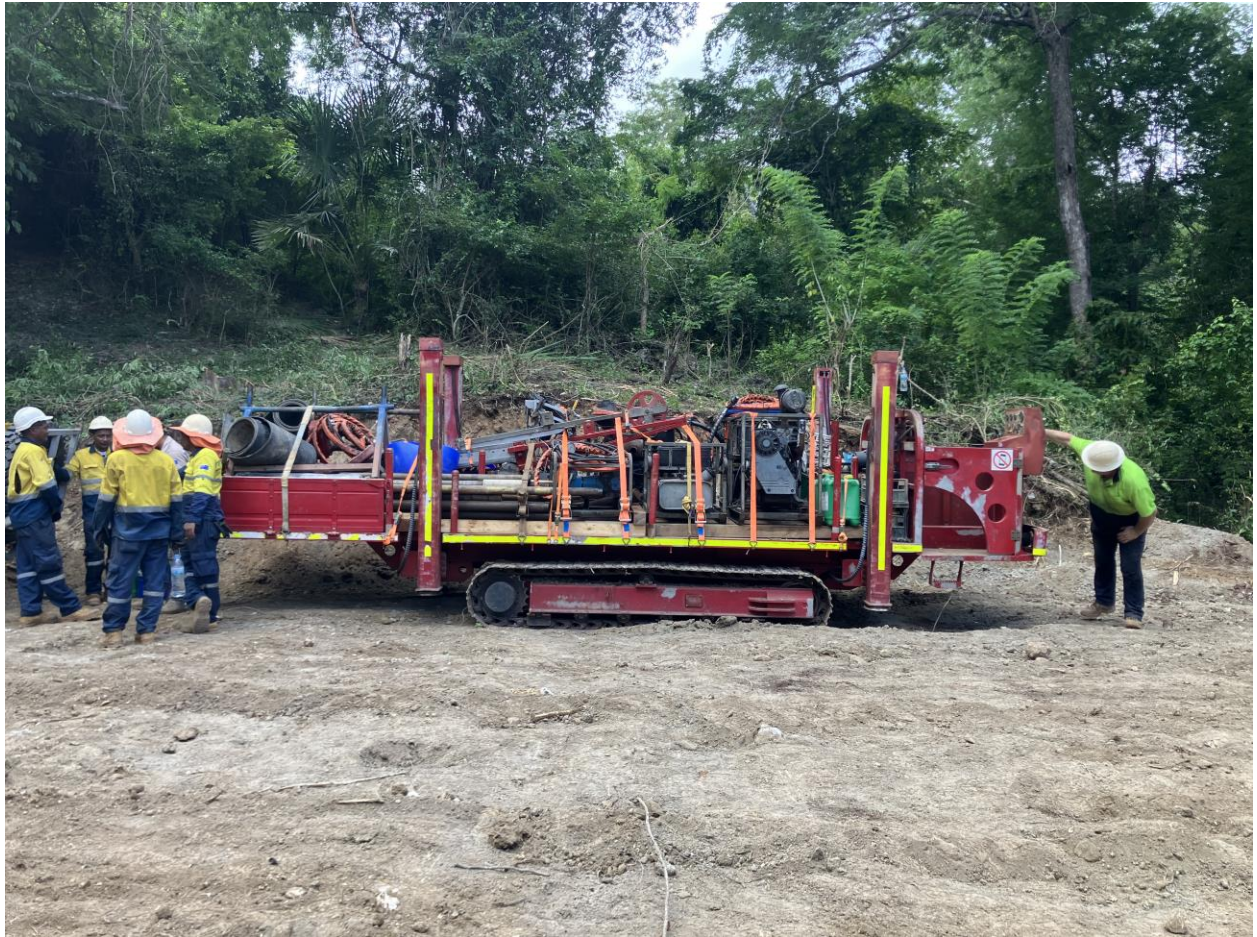
Figure 7: The portable diamond drill and ancilliary equipment parked on the first drill site at Ira Miri
