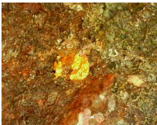
Figure 1 Close-up view of visible gold from sample ARK000678, a sample of brecciated and gossanous quartz vein which assayed 122.8g/t Au at Dodd’s prospect. Width of gold grain is ~1mm.
