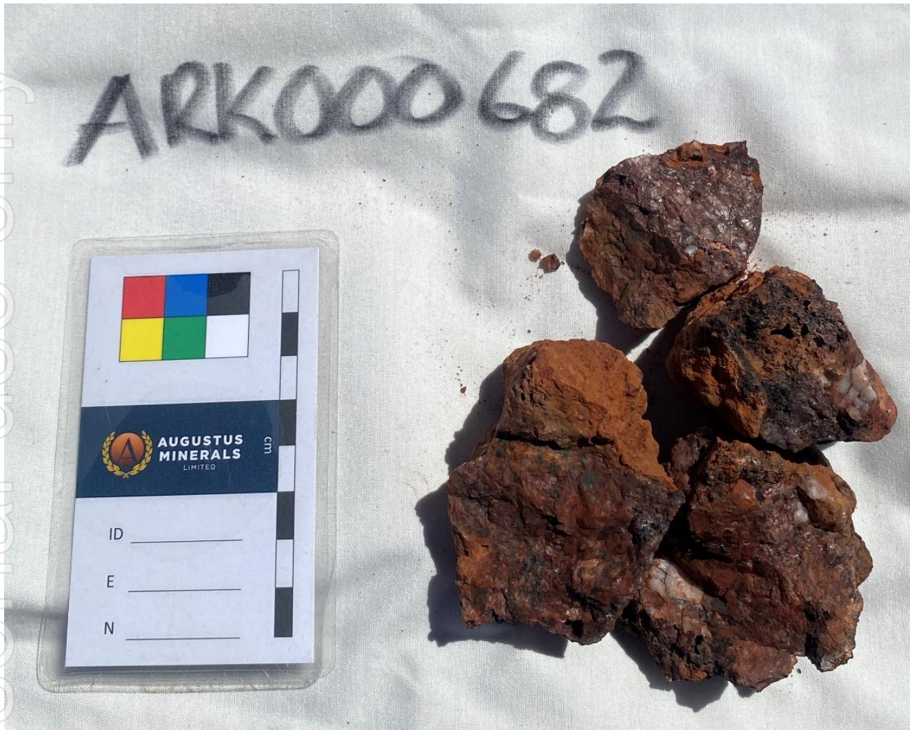
Figure 6 Rock chip of brecciated and gossanous quartz vein which assayed 29.0g/t Au at Dodd's prospect.
