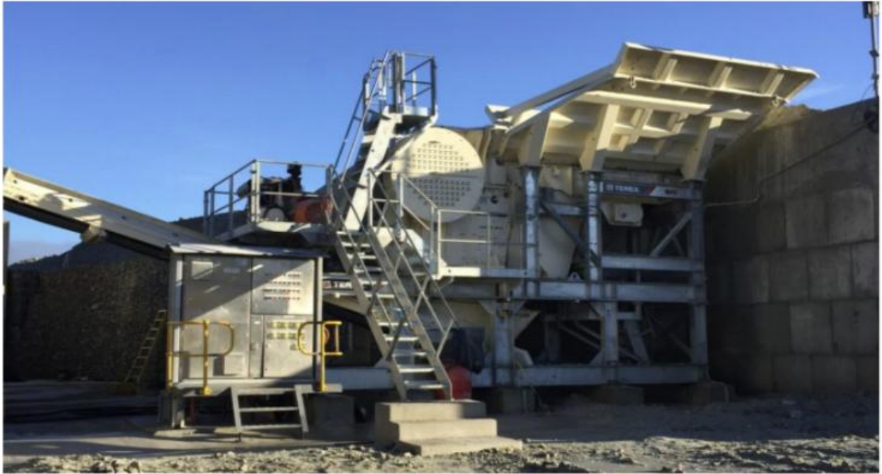
Figure A11: Example of the proposed modular Jaw Crusher
