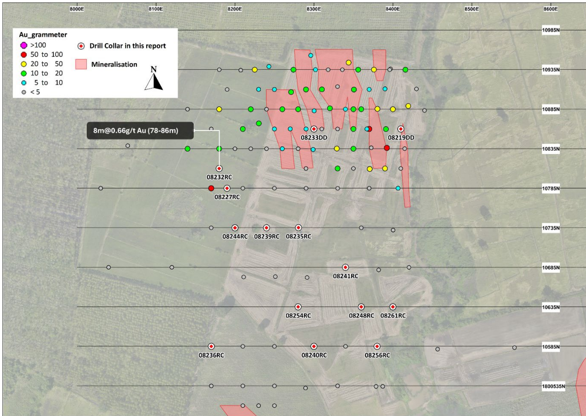
Figure 9: Drill hole locations 20 and gold assay highlights 21 , Northern Zone of Chatree South-East Complex.
