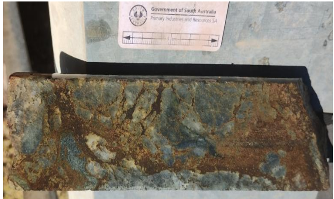
Figure 2a and 2b: Bedded Sulphides seen in BUDD192 (left). Sulphide breccia seen in BUDD192 (right).
