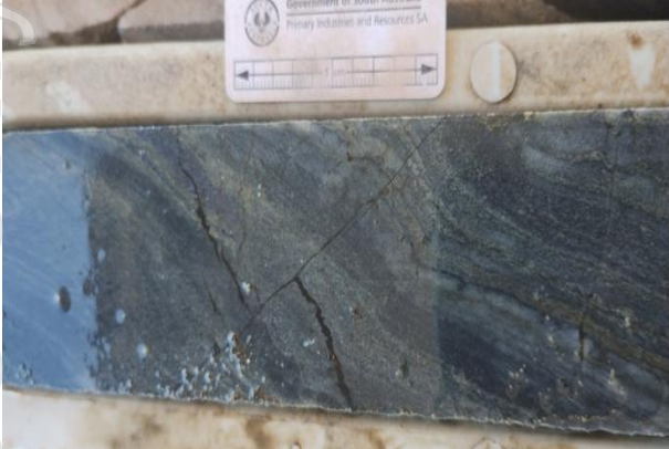
Figure 2a and 2b: Bedded Sulphides seen in BUDD192 (left). Sulphide breccia seen in BUDD192 (right).
