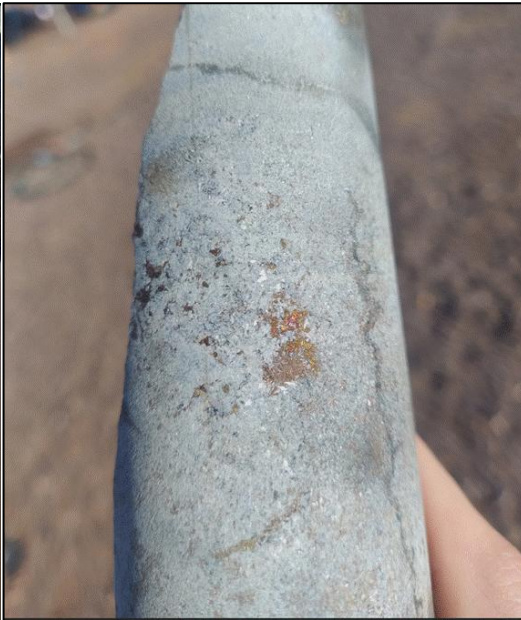
Figure 3a and 3b: Chalcopyrite and Pentlandite seen in cross-cutting veins in BUDD149 (left). Disseminated Bornite and Sphalerite in BUDD100 (right).
