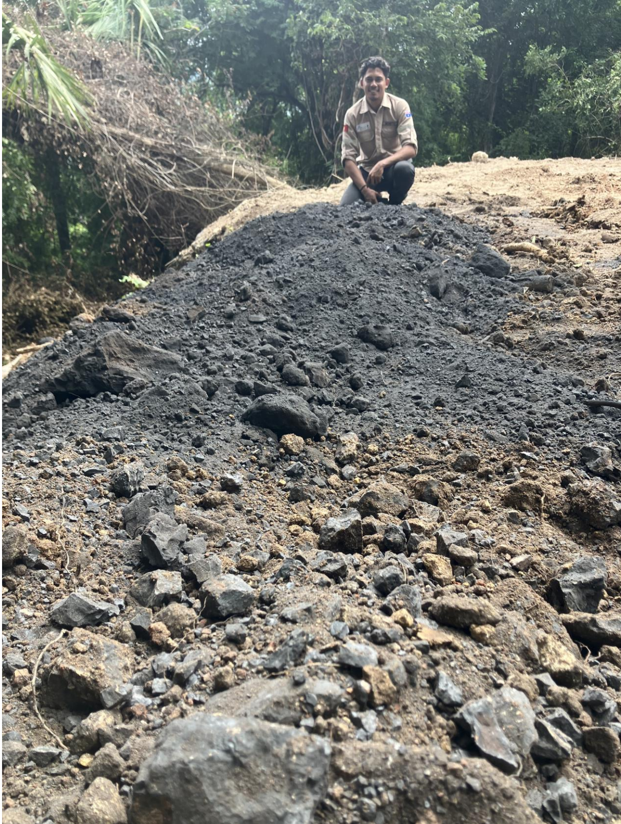
Figure 4: Estrella Exploration Geologist Bebeto Abilio looking over the first few buckets of massive manganese oxides from trench EMT01 which were uncovered just 0.7m below a well used footpath, with no surface expression evident
