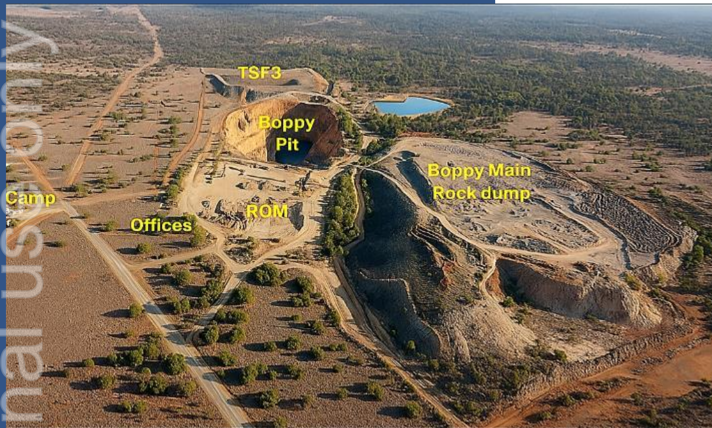
Figure: Aerial view of Mt Boppy Gold Mine looking south across the Main Rock Dump toward the Open Pit and TSF3 Tailings impoundment.
