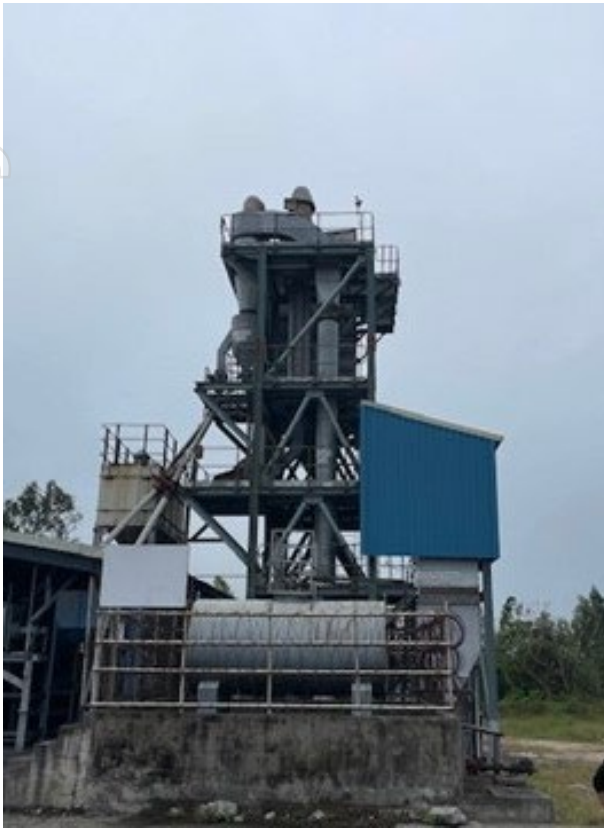
Figure 2 Graphite concentrate dryer
