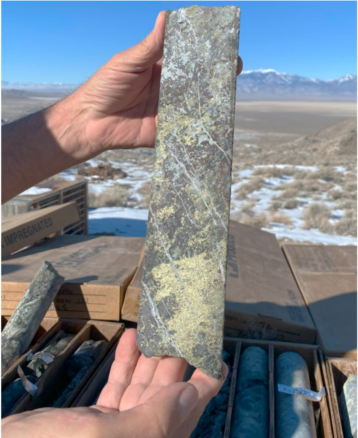
Figure 3: Drill core from WD22-01C from between 421.21-425.33m downhole (3.4% Cu, 91g/t Ag, 0.74g/t Au, 17g/t In, 0.05% Mo - See ASX announcement dated 19 September 2023: Assays Confirm Growth Potential at West Desert). This intersection is located outside of the current West Desert MRE.
