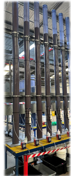
Oxide and Transitional Heap Leach Column Tests recently completed with excellent results
