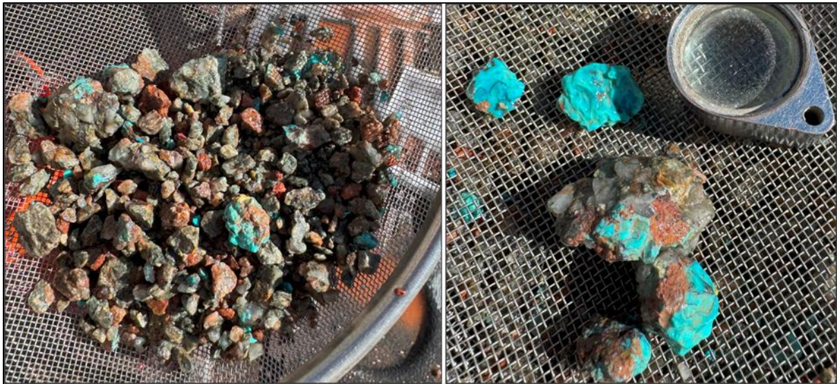
Figure 1: Copper carbonate associated with veining and intense alteration at Ford Prospect (PRC010. 256 ft to 260 ft)
