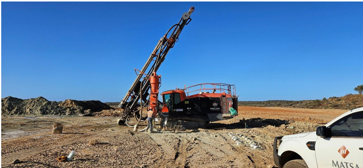
Plates 10 & 11 Grade control drilling on the West Lode (starter pit) at the Devon Pit Gold Mine
