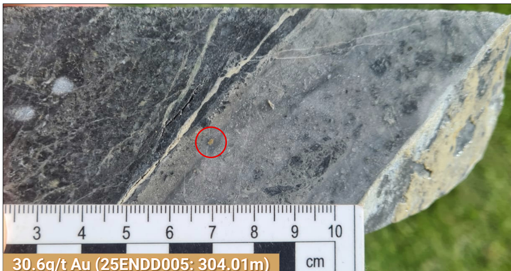
Photo 1. Sample photo of 25ENDD005 from 304m – 304.3m @ 30.6g/t Au with visible gold circled in red in a quartz-pyrite vein within moderately phyllic altered granite host rock.
