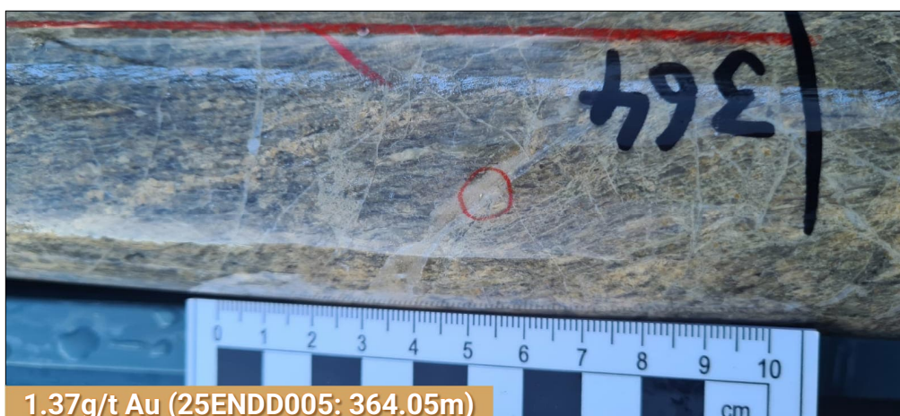
Photo 2. Sample photo of 25ENDD005 from 364m – 364.5m @ 1.37g/t Au with visible gold circled in red associated with quartz-iron carbonate-pyrite-arsenian pyrite +adularia veins in granite host rock.
