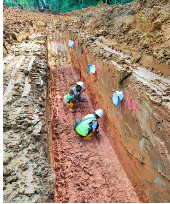
Little MacKenzie southern trench, Geological team preparing the base of the trench for channel sampling, collecting 2m wide channel samples (0.1 x 0.1 x 2 m) over the length of the trench
