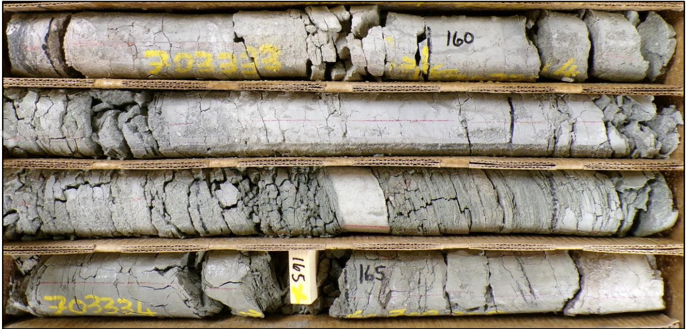
Figure 1. Clay-rich RMDD002 drill-core from 160-165ft (3,280ppm Li) used in Falcon beneficiation testwork.
