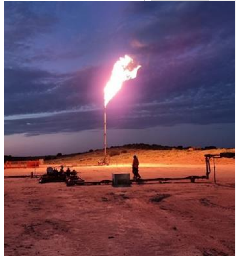
Figure 1: Gas flare from Kiwi-1 wellsite at 1.7 mmcf/d
