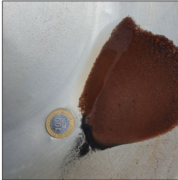
Figure 7: Fine grained HM concentrate from panned 1m channel sample from the GRMGB0002 locality. The visual representation of heavy mineral (HM) and rutile mineralisation shown in this release is based on preliminary visual reconnaissance with no sampling results. Assay results are pending and have not yet been verified through laboratory analysis. Investors are cautioned that the information is indicative only and should not be relied upon as a definitive measure of mineralisation or economic potential. Further exploration and analytical testing are required to confirm the extent, grade, and economic viability of the mineralisation.
