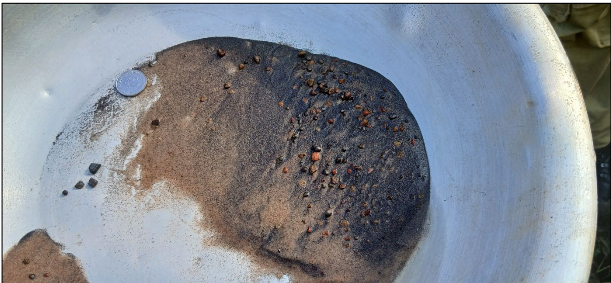
Figure 6: Fine grained HM and rutile grains/nuggets (1-5mm) from panned concentrate of a grab sample from the site shown in Figure 5 (GRMGRA0001). The visual representation of heavy mineral (HM) and rutile mineralisation shown in this release is based on preliminary visual reconnaissance with no sampling results. Assay results are pending and have not yet been verified through laboratory analysis. Investors are cautioned that the information is indicative only and should not be relied upon as a definitive measure of mineralisation or economic potential. Further exploration and analytical testing are required to confirm the extent, grade, and economic viability of the mineralisation.
