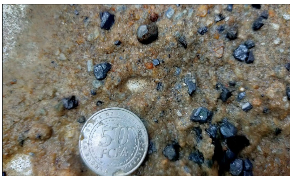
Figure 10: Coarse rutile nuggets from panned stream sediment concentrate from site GRMST0001. The visual representation of heavy mineral (HM) and rutile mineralisation shown in this release is based on preliminary visual reconnaissance with no sampling results. Assay results are pending and have not yet been verified through laboratory analysis. Investors are cautioned that the information is indicative only and should not be relied upon as a definitive measure of mineralisation or economic potential. Further exploration and analytical testing are required to confirm the extent, grade, and economic viability of the mineralisation.
