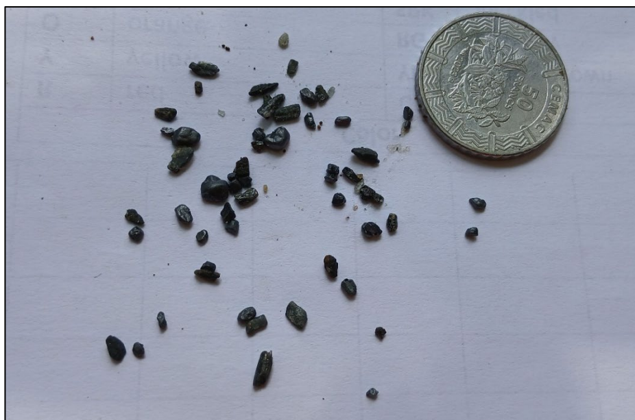
Figure 9: Coarse rutile nuggets (1-5mm) from GRAMAU0004. The visual representation of heavy mineral (HM) and rutile mineralisation shown in this release is based on preliminary visual reconnaissance with no sampling results. Assay results are pending and have not yet been verified through laboratory analysis. Investors are cautioned that the information is indicative only and should not be relied upon as a definitive measure of mineralisation or economic potential. Further exploration and analytical testing are required to confirm the extent, grade, and economic viability of the mineralisation.
