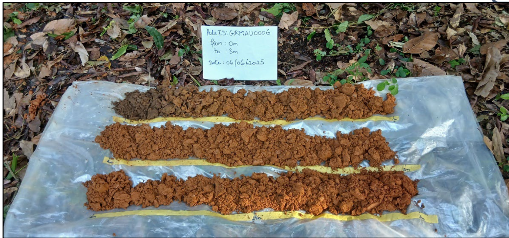
Figure 3: One meter hand auger samples laid out next to the drill site (from hole GRMAU0006).
