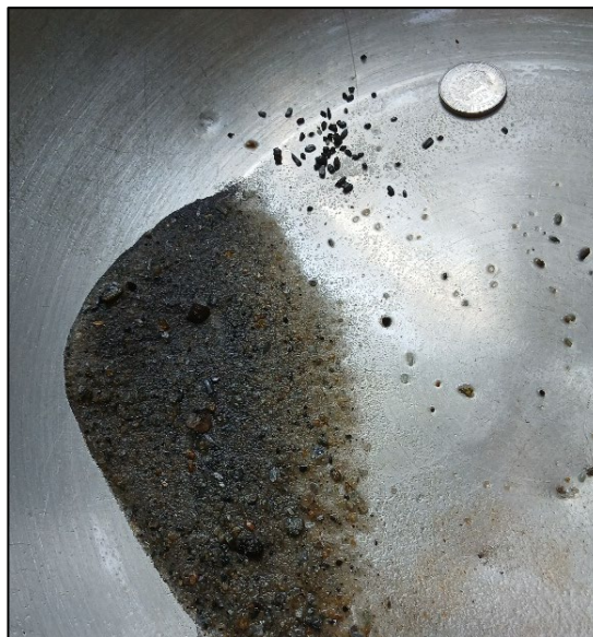
Figure 8: Fine grained HM and rutile nuggets grains (~1mm) from panned concentrate of 1m samples from the GRMAU0004 auger hole. The visual representation of heavy mineral (HM) and rutile mineralisation shown in this release is based on preliminary visual reconnaissance with no sampling results. Assay results are pending and have not yet been verified through laboratory analysis. Investors are cautioned that the information is indicative only and should not be relied upon as a definitive measure of mineralisation or economic potential. Further exploration and analytical testing are required to confirm the extent, grade, and economic viability of the mineralisation.
