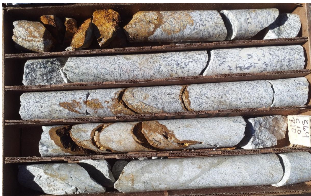
Figure 1 - Argillic altered and veined (qtz-sulphide) granite from drill hole GDD02 where samples were taken for mineralogical study. The rock is composed of quartz (56%), k-feldspar (26%), muscovite (7%) and kaolinite (5%).
