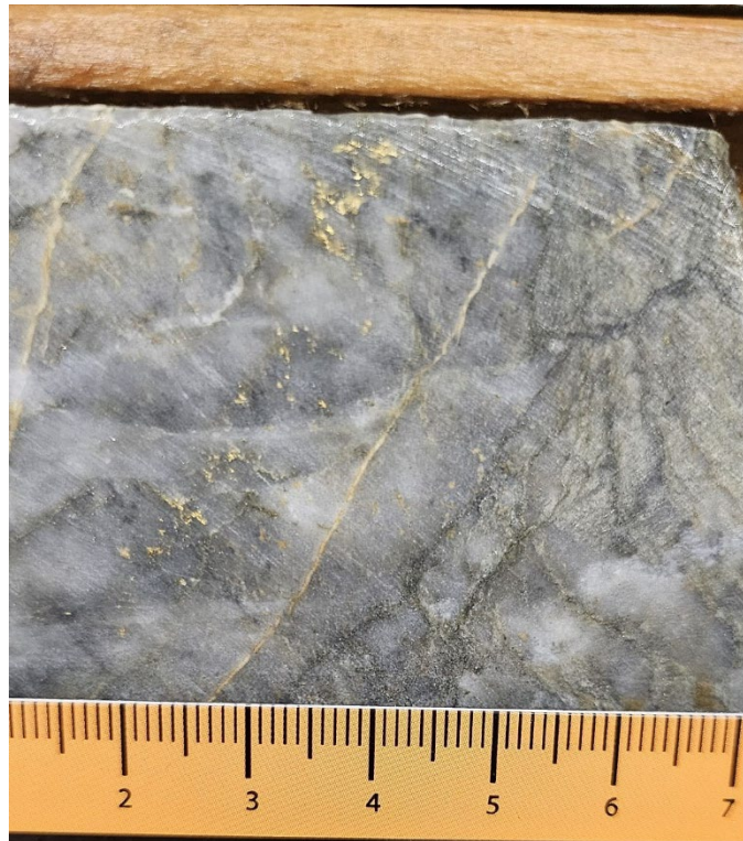
Figure 3: Photo of core from drillhole BO-21-08 at the Paquin Prospect showing visible gold within characteristic blue-grey quartz (184.5m). Scale unit is centimetres. The one metre interval 184-185m assayed 1m@ 129.25g/t Au, within 9m @ 16.96g/t Au from 178.5m 8
