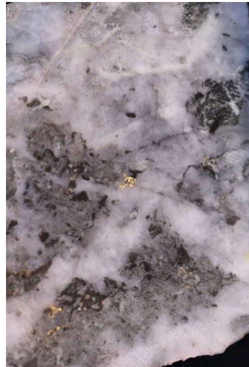
NSD057 – 108.2-109m includes multiple instances of visible gold (VG) in quartz veining. This is not typical for Stawell – and the geology, mineralisation and structure have strong similarities to the historic Mariners mines that boasted an historic production grade of ~30 g/t Au (see p. 11 for details on Mariners).
