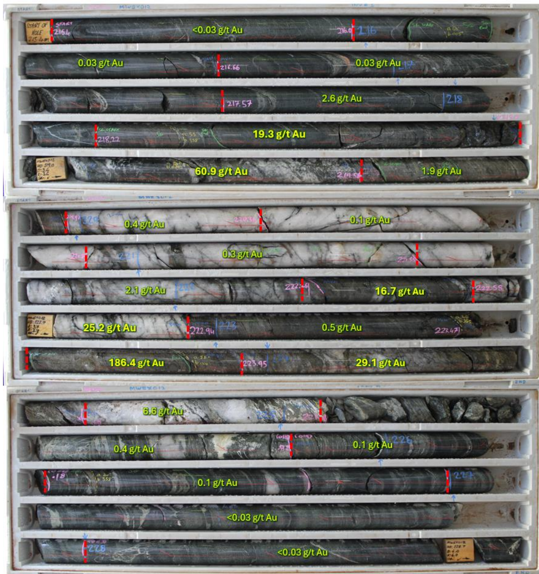
Figure 2 Photo of core from MWEX012 with Au grade and interval displayed on the core photo
