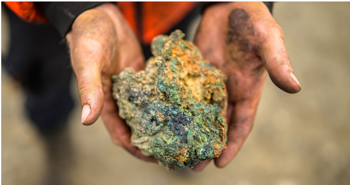
Figure 5: Copper gossan from the Hailstorm Prospect. This is massive chalcocite (copper sulphide) and returned a laboratory assay grade of >50% Cu, 61g/t Ag (Sample Y007193, 50% Cu is the upper limit of the assay technique used).
