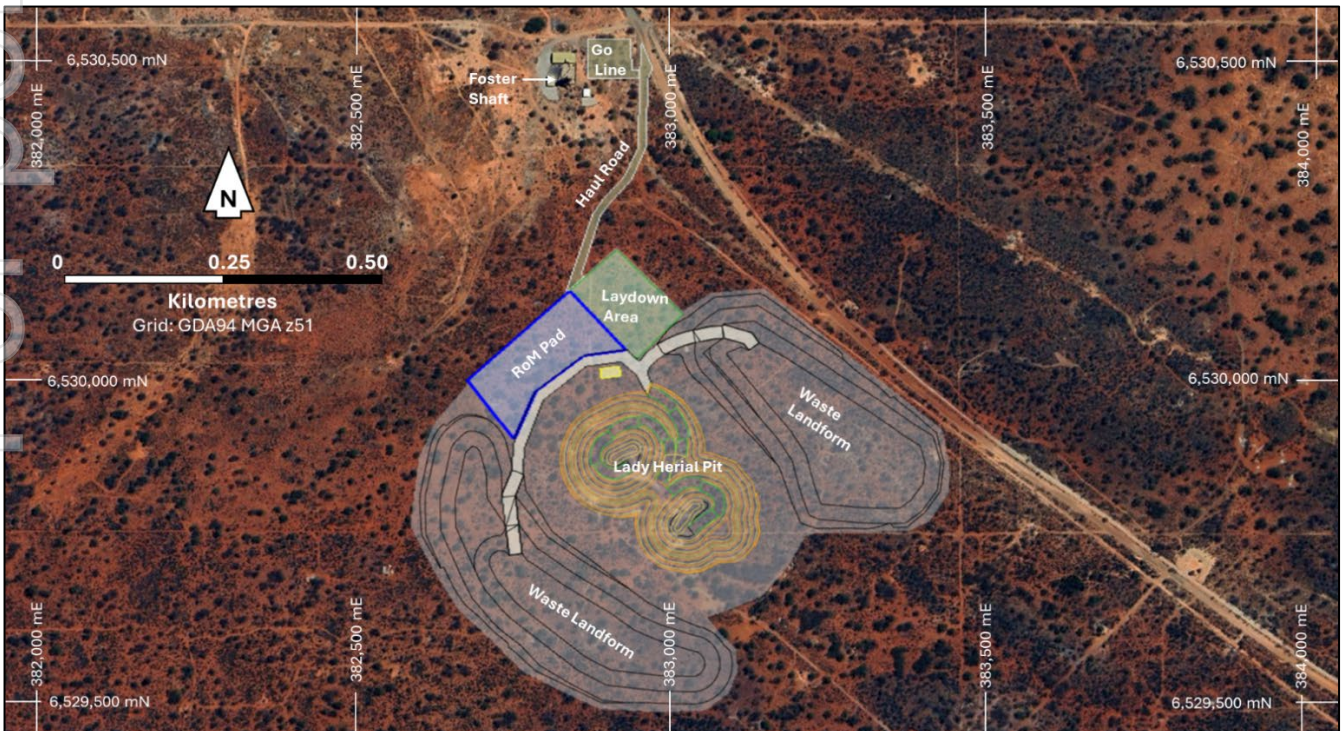
Figure 13: Lady Herial development and open pit mine design layout.
