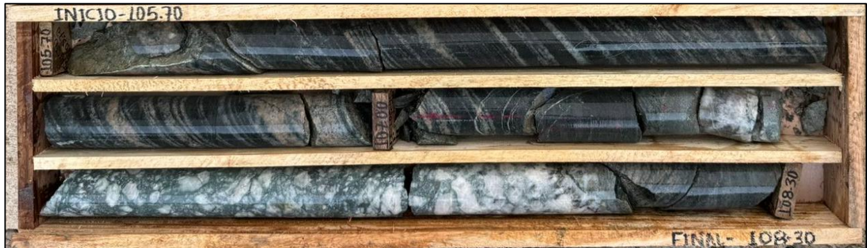
Photo 2. Target mineralized vein #1 (DDH SB-25-01, from 105.7 to 108.3m) intersected under the main Santa Barbara development tunnel (Figures 1 and 2). The vein is comprised of an early quartz and semi-massive pyrite that (almost 50% of the stage 1 vein event) is visible on the vein edges, following right-lateral fault zones. This event is followed by an epithermal reactivation manifested in breccia textures affecting the initial stage and a second generation of quartz and calcite fragments cemented by chlorite and sericite/pyrite alteration haloes in the wallrock clasts. Iron poor yellow sphalerite and coarse galena complete the epithermal paragenesis. Assay results are pending.
