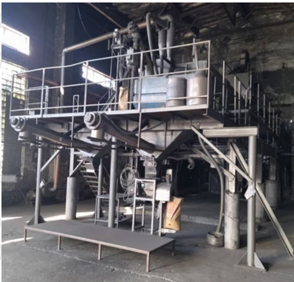
Figure 1 – High Purity (99.5%) Graphite Production Line at Zavalievsky Graphite
