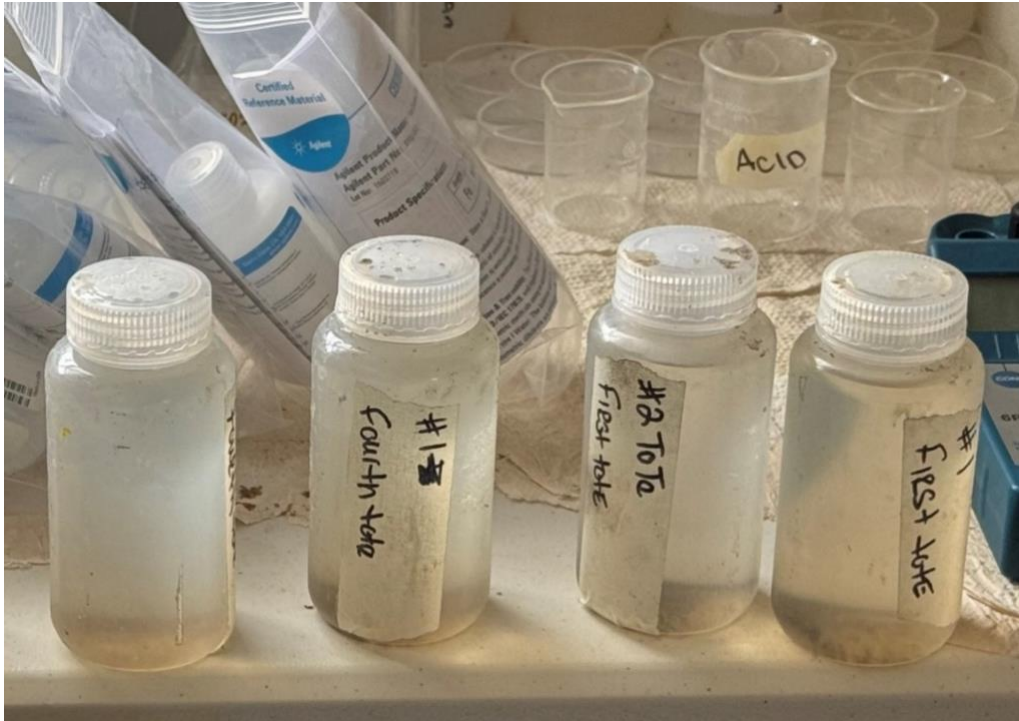
Figure 1: The swabbed brine samples from the Bosydaba#1 well in May 2025 after clean-up of aquifers.
