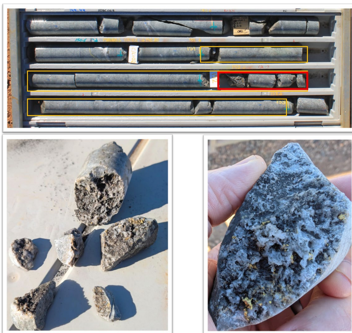
Figure 2: [TOP] shows the core from RDRC068, 149.44m to 153.13m, the yellow box highlights the interval 2m @116.3g/t from 151m to 153 m. The red box highlights the interval 0.2m @ 1,148 g/t Au from 152m-152.2m. [BOTTOM_LEFT] shows some core pieces from 152m-152.2m. [BOTTOM_RIGHT] shows a close-up of one of the pieces of core from the Bottom-Left figure with visible gold.
